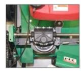
New single speed rear selfpropelled is great in hilly turf applications (KV650SPH)
