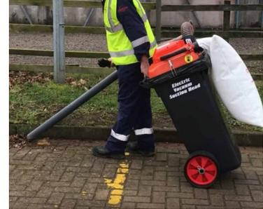
It is ideal for cleaning confined and awkward areas which cannot be accessed with mechanical sweepers. The litter does not pass through the impeller allowing broken glass to be collected. This machine is excellent for collecting small material such as smoking related and confectionery litter.
