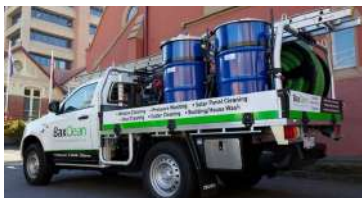
Single cab alloy tray ute with dual 205L drums & tippers
