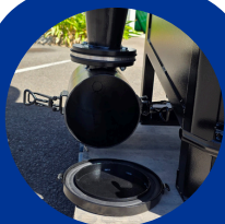
CYCLONIC DUST SEPARATOR WITH DUST KNOCKOUT BOX
